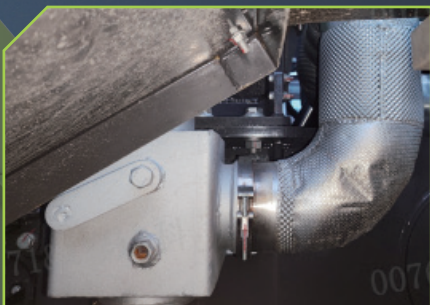
Thermal insulation tile for exhaust pipe
